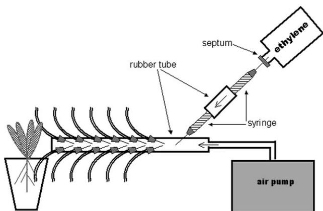
**Fig. 1.** System used for the application of ethylene to plants. For details, see Materials and methods.
